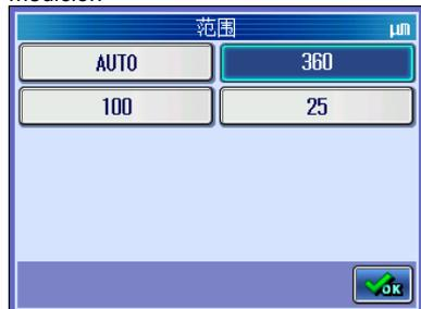
**2** Seleccione un margen de medición utilizar y pulse
