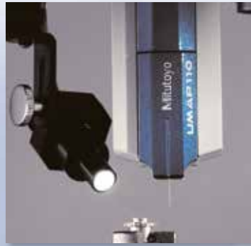
Highly accurate height measurement thanks to image auto-focus
