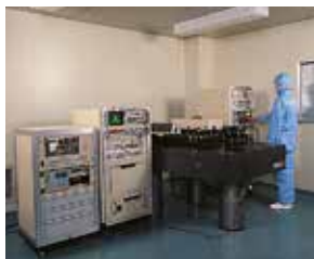
Iodine absorption stabilised He-Ne (633 nm) laser for length measurement
