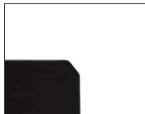
Chamfered part of a machined surface
