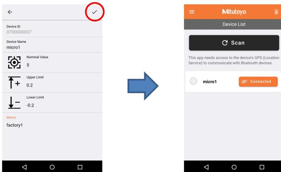
The screen displayed in "Measure" changes when tolerance settings are made. They are displayed in green when they are within the tolerance range and in red when they are outside the tolerance range. If you have registered multiple entries, you can check them all on the "All" screen.
