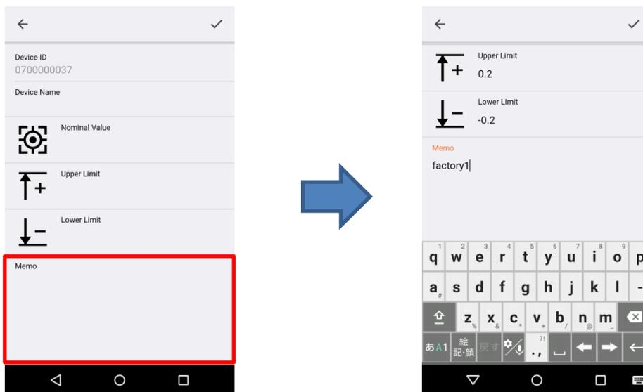
⑧ After entering the setting, tap "✓" in the upper right of the screen to complete the setting.
