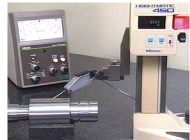
The three-point method, which utilizes an indicator and V-block, offers better resolution but is not sensitive to common lobing conditions.
