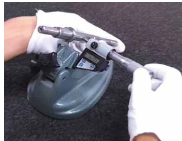
Diameter measurement using a micrometer cannot detect an odd-number lobing condition, and the resolution is limited.
