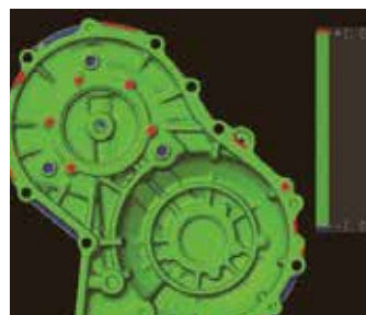
3 lines at 120° capture internal shapes in a single run.
