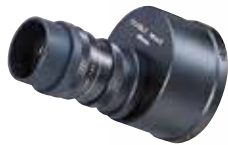
No. 375-044 Aids accurate measurement of hole-to-hole distances, hole diameters and sections using the double image generate when the feature under inspection is not aligned with the optical axis of the microscope. • Magnification: 10X • Field number: 22
