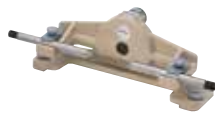
No.172-197 A tilt angle of \pm 10^\circ can be supported. Minimum reading of angle: 1^\circ Maximum support size: \phi 80 \times 140\text{mm}/3.15'' \times 5.51'' in horizontal orientation \phi 65 \times 140\text{mm}/ 2.56'' \times 5.52'' at a tilt angle of 10^\circ Mass: 2.5kg/ 5.51lb * Stage Adapter A is required.
