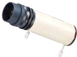
No. 375-043 Measures angle between workpiece edges by successive alignment with two crosshairs whose separation is adjustable and calibrated through 360° • Field number: 21 • Resolution: 5'
