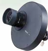
No. 176-357 Uses a template to superimpose screw thread forms (metric UST, Uni-field Screw Thread), concentric circles, and crosshairs on the workpiece image for quick and efficient measurement by comparison. • Magnification: 10X • Field number: 21
